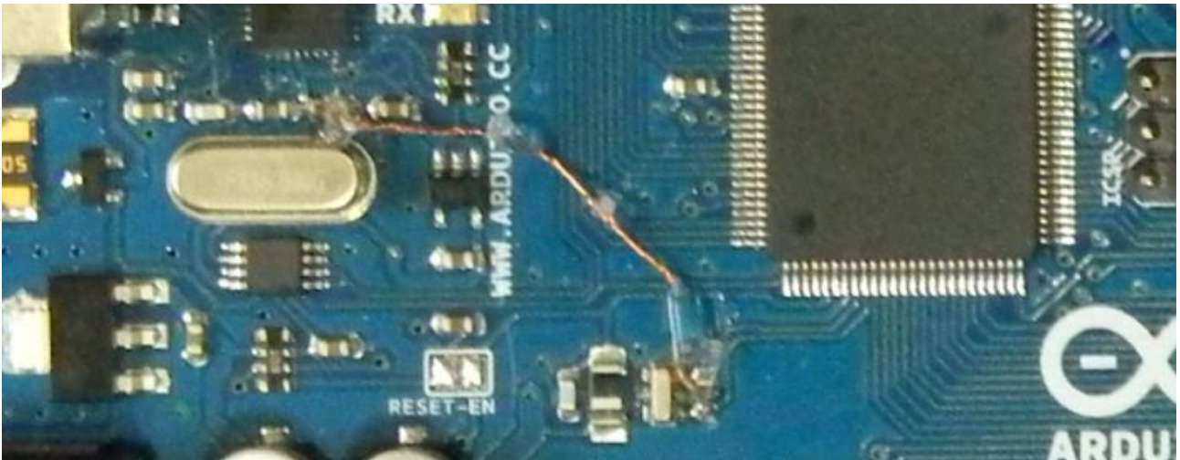
Figure 5: ArduinoMega2560: synchronising main \mu C's and USB2serial's (Atmega8U2) clocks
