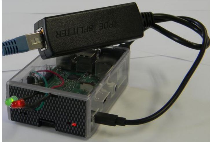
Fig. 8: Power over Ethernet splitter 5V, 2A
