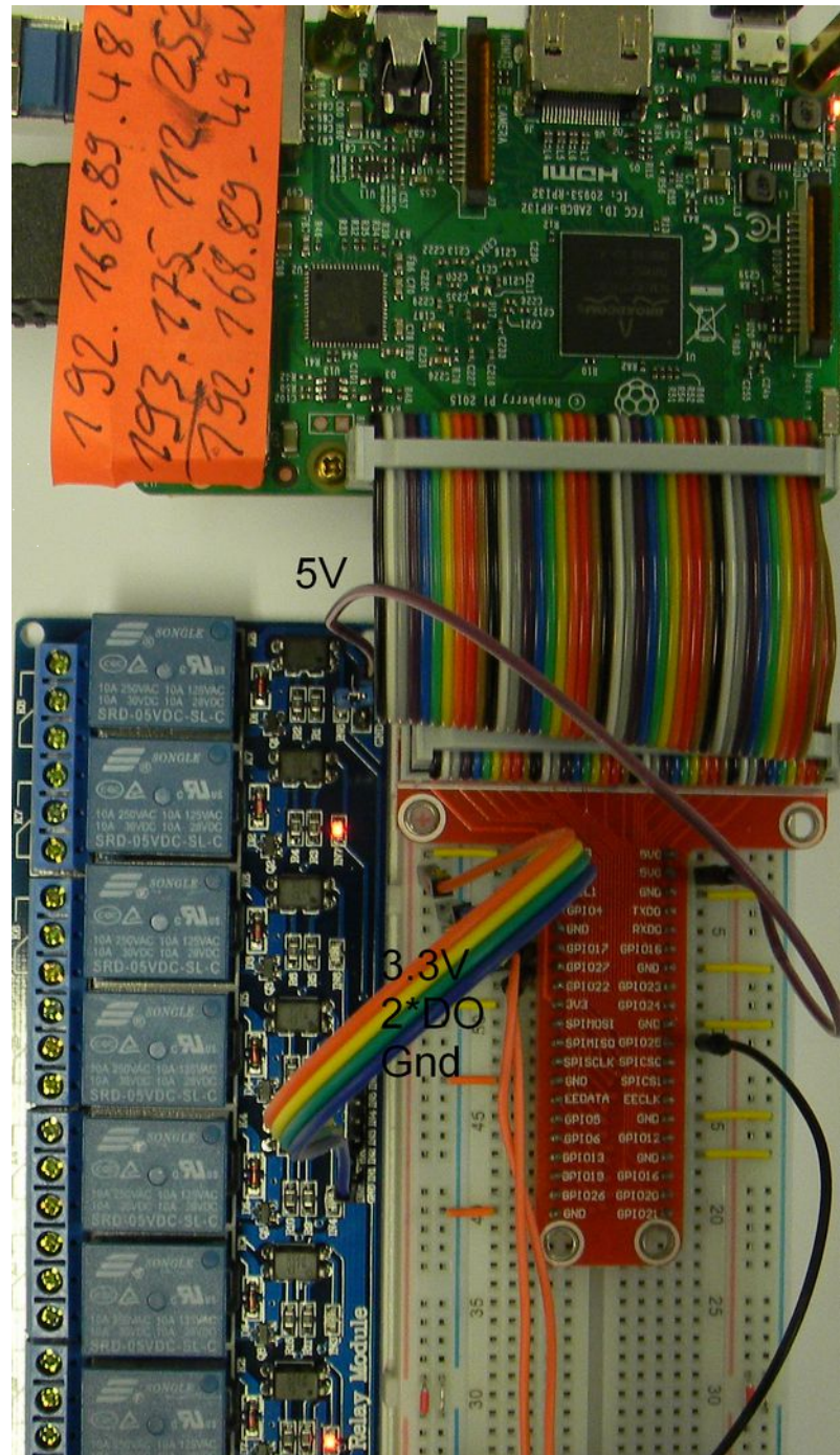
Fig. 6: Eight relays module 10A
