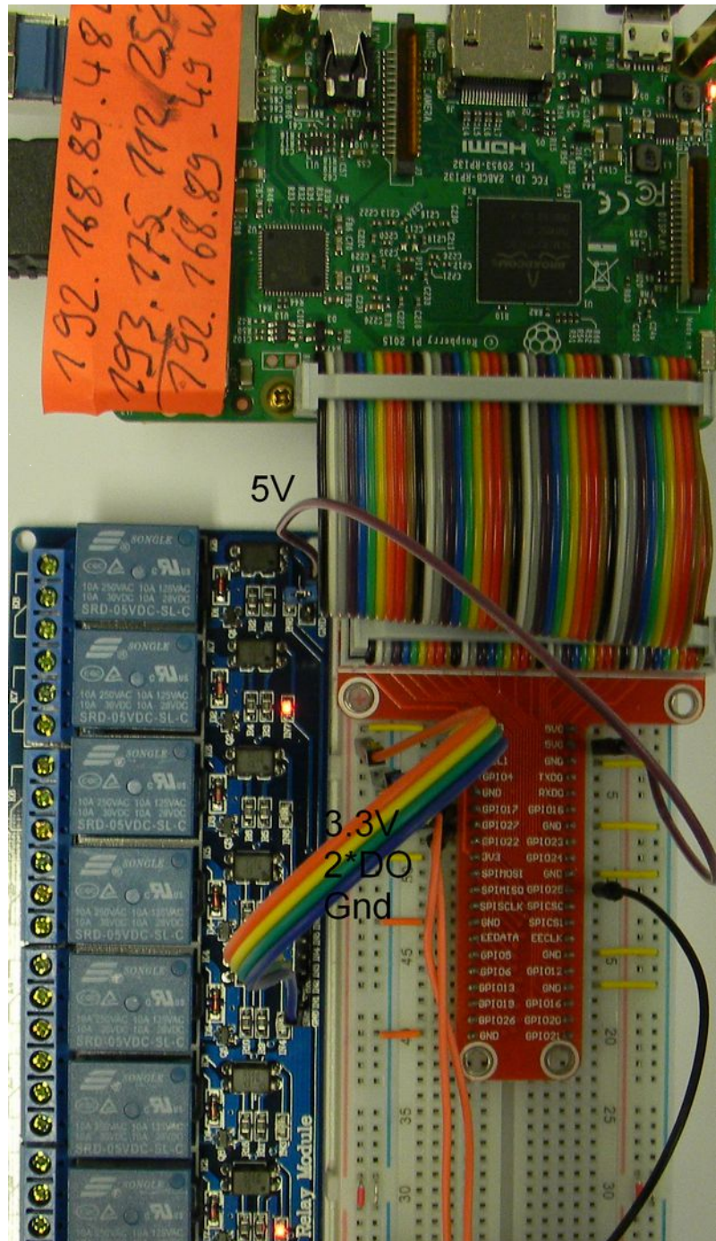
Fig. 6: Eight relays module 10A
